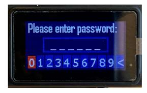
Enter the password using the [P] + [FN] buttons, [P] moves left and [FN] moves right, press the record button to confirm the highlighted password number. Proceed to enter the 6 digits of the password and the camera will automatically bring you to the User List.
