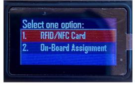
To select an option, use the [P] + [FN] button to navigate up and down. Use the record button to hit enter.
